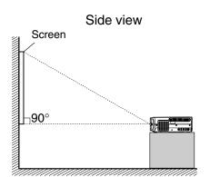
Point the lens straight at the center of the screen as above.
